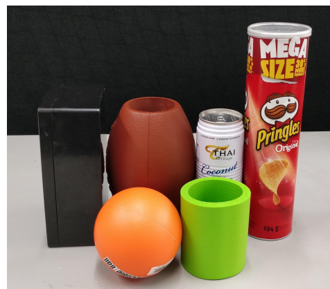
Fig. 4. Objects used for our robot experiments, from left to right (objects, surface properties): plastic box (planer, smooth, rigid), plastic ball (spherical, smooth, rigid), football sleeve (spherical, rough, deformable), foam sleeve (cylindrical, smooth, deformable), metal can (cylindrical, rough, rigid), and cardboard can (cylindrical, smooth, rigid).
