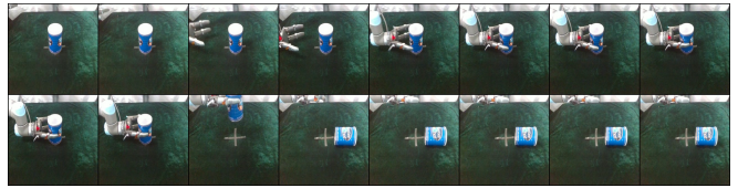
Fig. 2: Visualization of video frames from the front camera during a pickup task. Frames are visualized at every second starting from the top left and ending at the bottom right [6].
