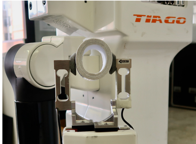
Fig. 1: Grasping an object with TIAGo’s sensorized parallel-jaw gripper.
